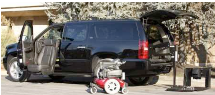
Figure 1: ATRS system integrated into a traditional Chevrolet Suburban. By integrating robotics and automation technologies, the need for a van conversion is eliminated.
