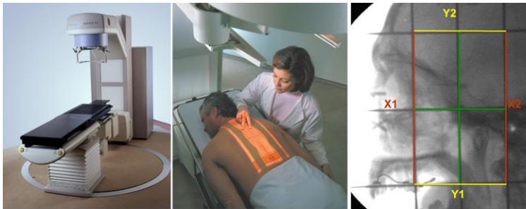
Fig. 2 LEFT: Physical device with imaging components; CENTER: Aiming, shaping a radiation beam by projecting a light field onto the patient's skin. RIGHT: Simulation image of a lateral head field with beam info superimposed.
