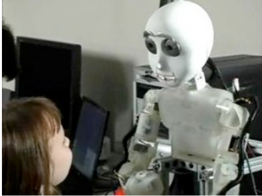
Figure: Our child-sized humanoid robot (which works from a desk top or on a mobile platform) interacting with a child, part of the research toward robots that can help in the education and socialization of children with special needs.
