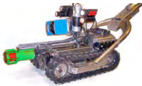
Responder™ Pipeline Robot
